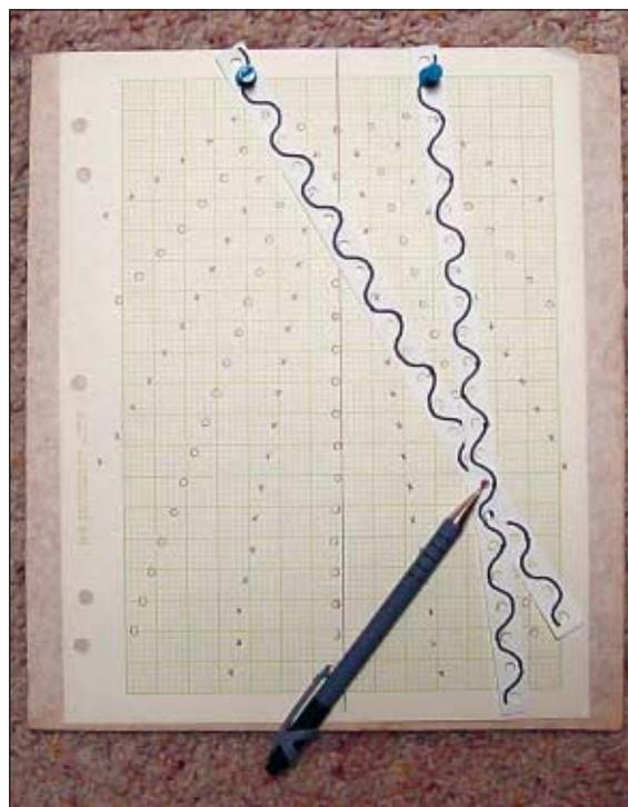
**Fig. 1. Photograph shows a completed set of nodal and antinodal lines created by aligning the holes of two pin-feed strips. Antinodes are marked with circles; nodes are marked with x's. The variation of pattern spacing with source separation can be studied by this method. Wavelength can also be changed to other multiples of the ½-in hole spacing.**
